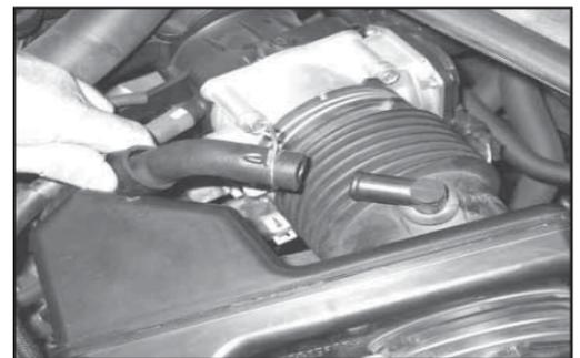
10. Release the clamp that secures the crank case vent hose to the stock intake tube and remove the crank case vent hose as shown. Loosen the clamp that secures the stock intake tube to the throttle body.
