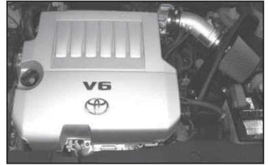
35. Reconnect the vehicle's negative battery cable. Check to ensure all hose clamps and fittings are properly tightened and positioned correctly before starting the vehicle.
