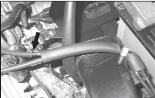
31. Connect the open end of the vacuum line installed in the previous step to the stock fitting as shown in the photograph.
