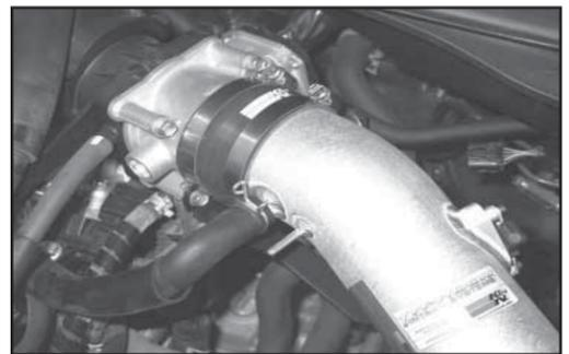
25. Connect the crank case vent hose to the fitting on the K&N® intake tube; secure with the factory spring clamp.
