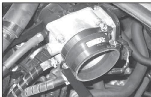
20. Install the provided silicone hose (084031) onto the throttle body and secure with the provided hose clamp.
