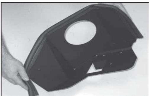
15. Install the edge trim onto the heat shield.
