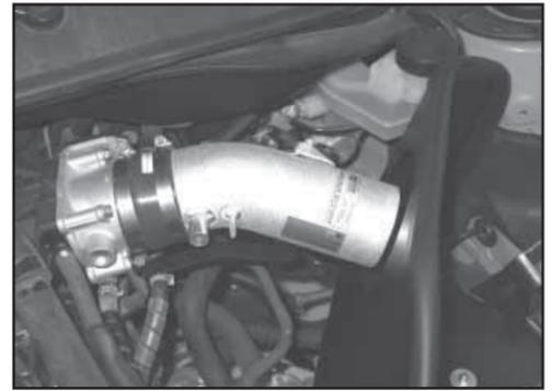
23. Install the K&N® intake tube into the silicone hose installed onto the throttle body in step # 20. Align the K&N® intake tube with the intake tube mounting bracket installed in step # 19. Secure silicone hose with provided hose clamp and mounting bracket with provided hardware.
