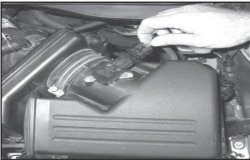
2. Disconnect the mass sensor electrical connection by depressing the center tab and gently pulling the harness away from the mass air sensor. Release the two wiring harness clips from the air box lid.
